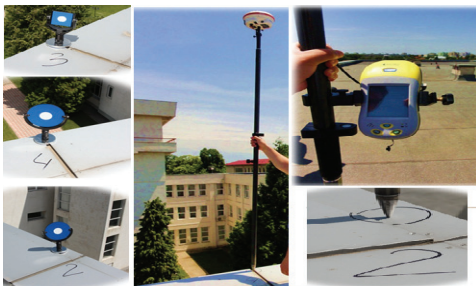
Figure 1. Measuring the coordinates of the HDS targets on top of the building
