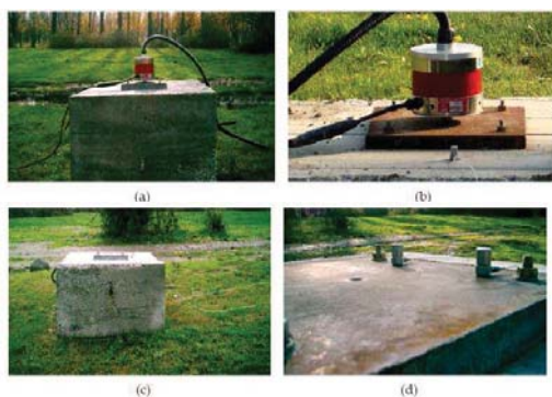
Figure 5. Electrodynamic shaker and accelerometer rests on a foundation: a) electrodynamic shaker placed on foundation; b) electrodynamic shaker and accelerometer positioned on the foundation, c) Measurements made on the basis of the Foundation, d) Accelerometer rests on the foundation.
