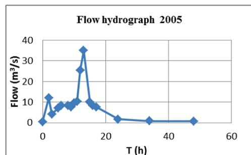
Figure 9. Flow hydrograph for flood event in 2005
