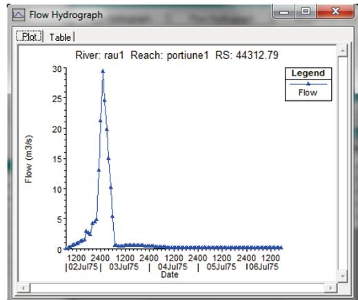
Figure 7. Flow hydrograph for flood event 1975
