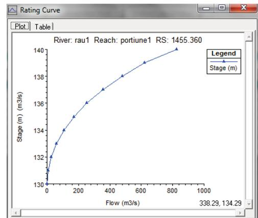
Figure 8. Rating curve used as downstream boundary condition
