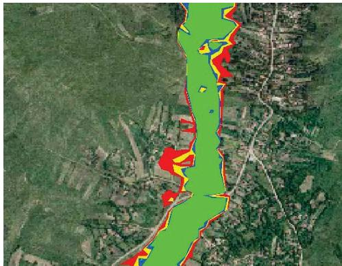
Figure 5. Detail of floodplain delineation where Q 10% - green, Q 5% - blue, Q 1% - yellow, Q 0,1% - red
