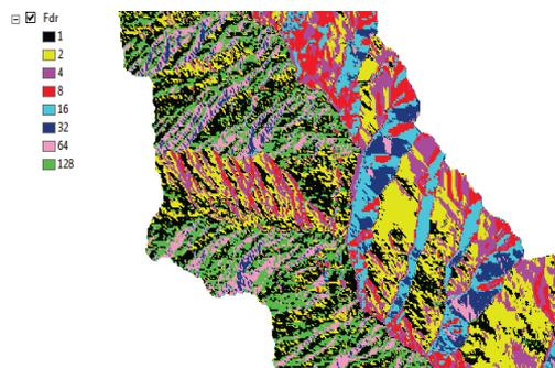
Figure 2. A closer view of flow direction raster with its legend
