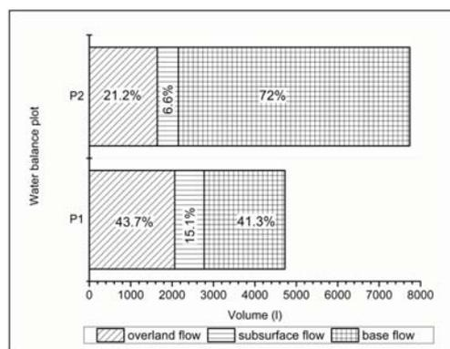
Figure 6. Total water volumes from water balance plots of grass covered (P1) and bare soil (P2) from 24/25.IV.2014
