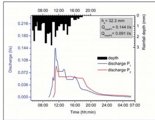
Figure 5. Hydrograph of overland flow from water balance plots grass covered (P1) and bare soil (P2) from 24/25.IV. 2014
