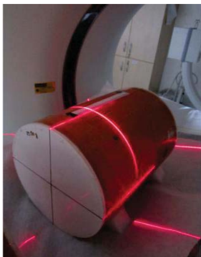
Figure 7. Scanning the soil sample
