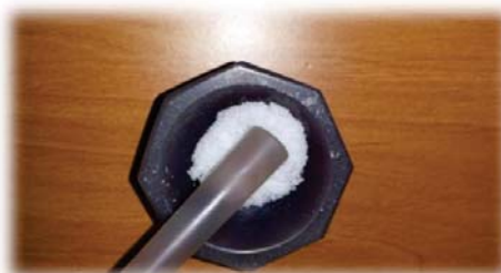
Figure 17. Grinding of KBr (potassium bromide)
