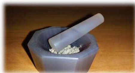
Figure 18. Grinding of the soil sample
