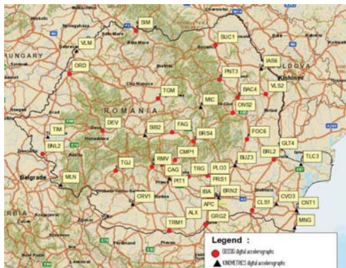
Figure 4. Distribution of Geosig and Kinematics digital accelerographs in Romania
