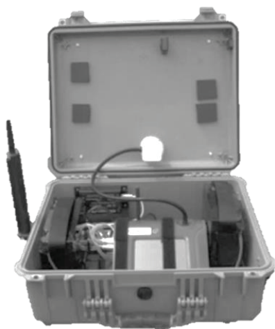
Figure 1. TSI DustTrak DRX 8533 particulate matter (PM) monitor, which allows the simultaneous measuring of various PM fractions i.e. PM 1 /submicrometric, PM 2.5 /fine, Respirable/PM 4 , PM 10 /Thoracic, and Total PM ( http://www.tsi.com )
