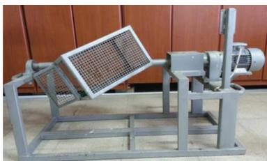
Figure 3. Durability tester for briquettes in experiments
