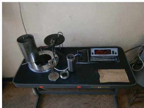
Figure 2. "CALORIMETER KL 11" - general view
