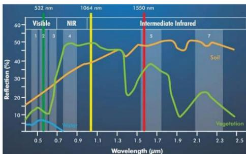
Figure 3. LiDAR wavelength sensitivities (Titan Brochure and Specifications, 2015)
