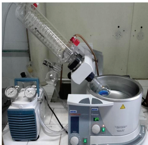
Figure 1. Rotary evaporator used for evaporation of extraction solvent
