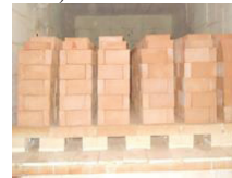
c) Burned bricks
