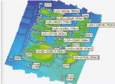
Figure 7. Stockpile volume computation using Agisoft Photoscan
