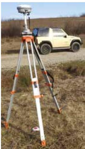
Figure 1. Dual band GNSS receiver - base station
