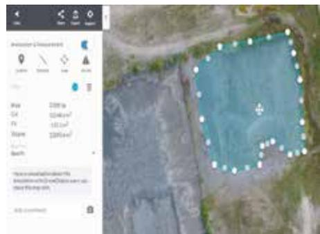
Figure 9. Stockpile volume computation using Dronedeploy
