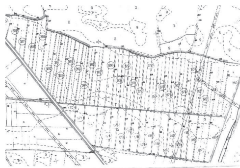
Figure 8. Technological parcelling of an area equipped with a drainage system
