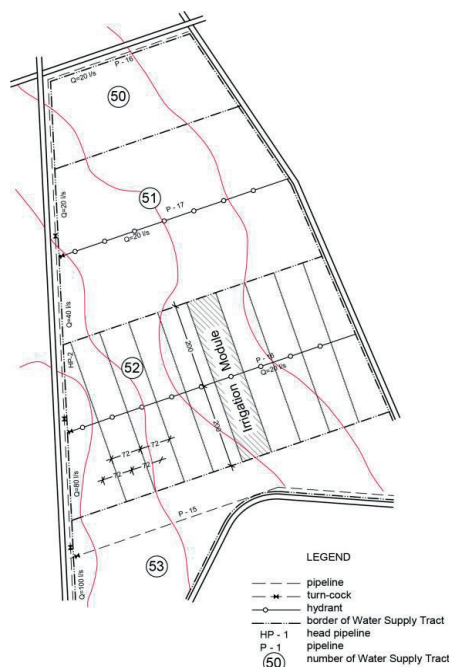
Figure 1. A scheme of structural land design in an area equipped with a subterranean pipe network with mounted hydrants
