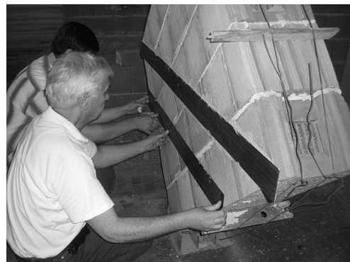
Fig. 14. Making specimens, by applying the Carbodur S 1012 strips
