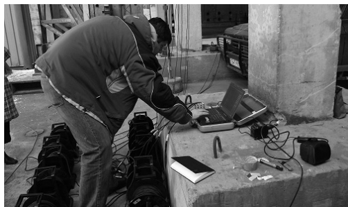
Fig. 3. GEODAS 12-USB, 12-channel seismic station, Buttan Service, Japonia
