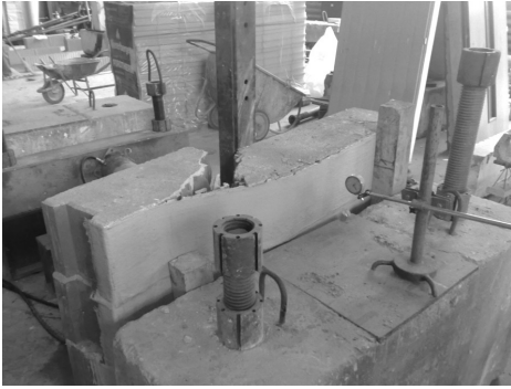
Fig. 17. The M30 model after failure
