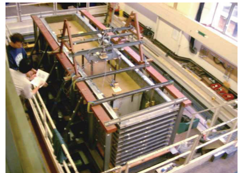
Figure 3. 3D model installed on the shaking table
