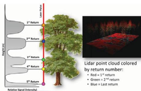
Figure 7. Multiple returns LiDAR pulses for determination of trees or crops height.
