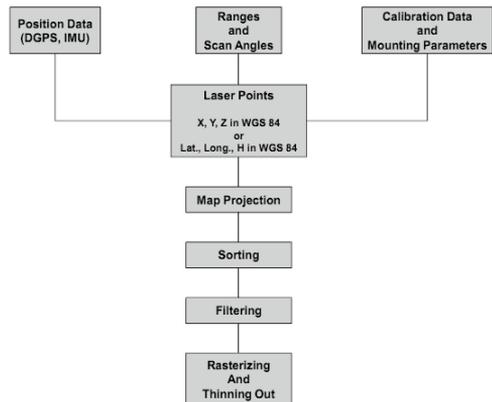
Figure 3. Diagram of the processes LiDAR data pass through before reaching the end user (ASPRS 2004)
