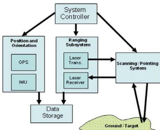
Figure 2. Diagram of a typical LiDAR system (NGA Standard, 2009).
