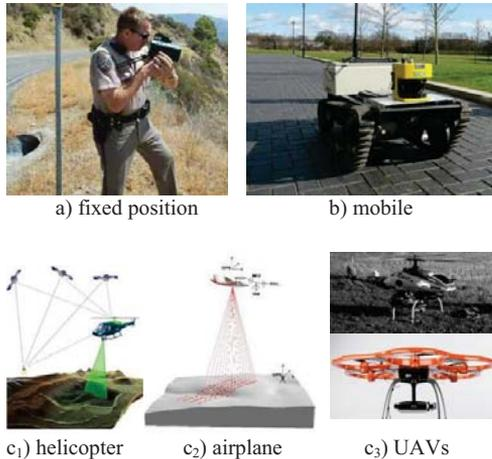
Figure 1. Types of LiDAR platforms
