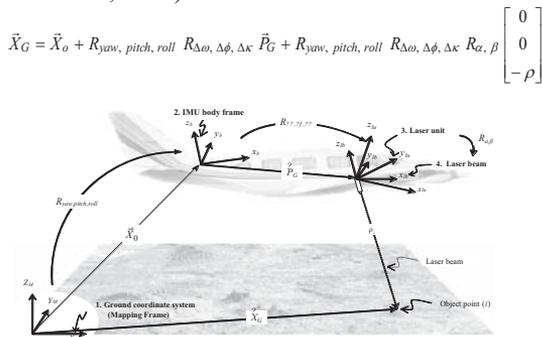
Figure 4. Relationship between LiDAR scanner, INS/IMU, GPS and their reference systems
