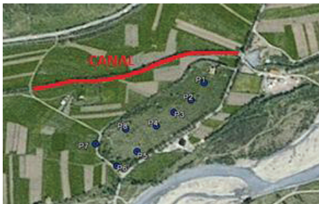
Figure 2. Layout plan of Voronet capture zone and of the artificial recharge canal
