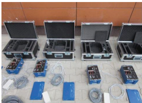
Figure 2. The data acquisition system with four GMS Plus digital seismic stations used for temporary seismic instrumentation of the new building of Biotechnology Faculty from Bucharest, B+G+2F (5 bays of 5.00 m and 5 openings of 5.00 m; H_{gf} = 3.80 m, H_1 = 4.10 m)
