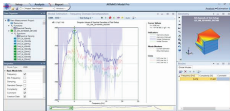
Figure 5. The results obtained using the Operational Modal Analysis, FDD technique
