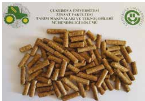
Figure 2. Pellets made from corn stems
