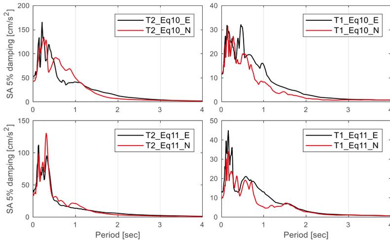
Figure 2. Acceleration response spectra at basement of buildings T1 and T2 on horizontal directions (N-S and E-W) due to earthquakes 10 and 11
