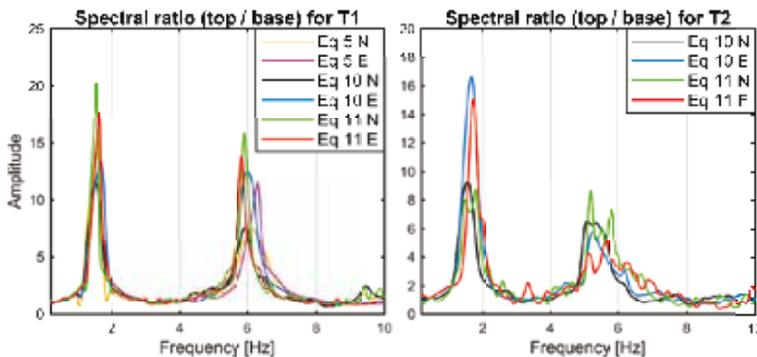
Figure 3. Spectral ratio for building T1 (left), for earthquakes 5, 10 and 11, and for building T2 (right), for earthquakes 10 and 11, on two horizontal components
