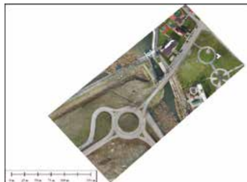
Figure 5. Orthophotoplan for the verified area at the resolution of 5cm/pixel
