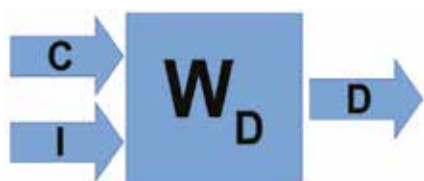
Figure 1. Model of experiment: W_D -process of obtaining HHO gas; C-concentration of electrolyte; I- force current power; D-gas flow
