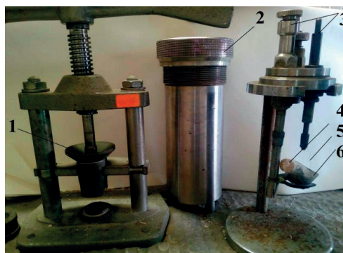
Figure 3. Equipment for the KL-11 calorimeter: 1-block press; 2-container of the calorimeter; 3-power electrodes; 4-block of combustible material; 5- kanthal resisting wire; 6-crucible
