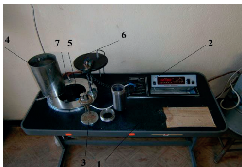
Figure 2. View of the KL-11 Mikado calorimeter: 1-working table; 2-meter; 3-fuel system; 4-outer casing; 5-vessel; 6-cover; 7-cooling part
