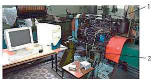
Figure 1. Experimental motor setup: 1 - D-243 diesel engine with the set of instruments; 2 - PC
