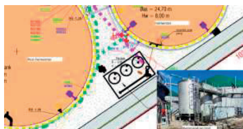
Figure 10. Digestate hygienization station
