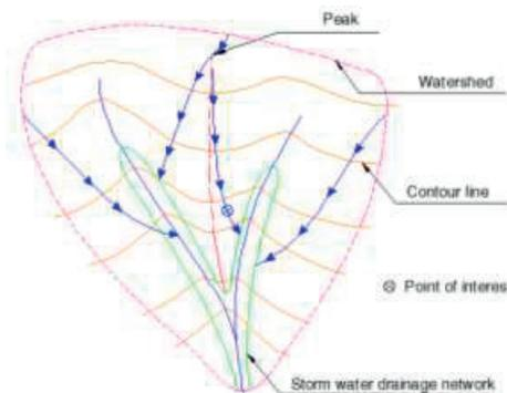
Figure 1. Determination of parameter “length of flow on versants” in model USLE
