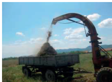
Figure 2. Shredding of plant residues of Rosa damascene Mill with silage harvester KPI-2,4
