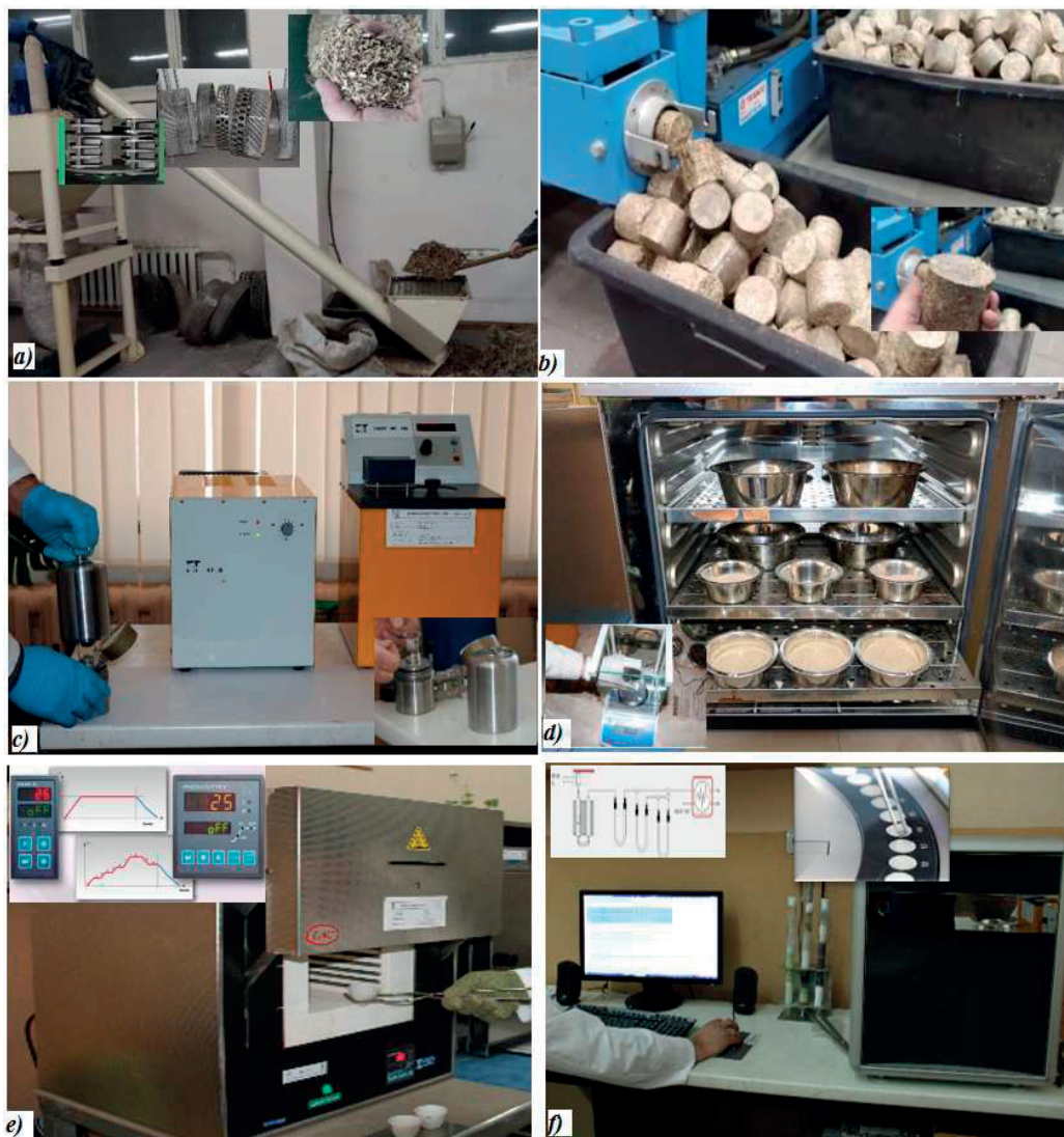
Figure 1. The pictures taken while preparing and testing the samples of Silphium perfoliatum : a) Grinding of the raw material; b) Biomass densification process; c) Determination of the calorific value of the studied samples; d) Determination of moisture content; e) Determination of ash content; f) Chemical analysis of the sample at the Vario MACRO cube CHNS and Cl elemental analyzer
