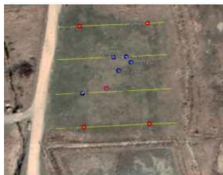
Figure 1. The position of the geotechnical boreholes (red points - existing boreholes, blue points - blocked boreholes) (Google Earth)
