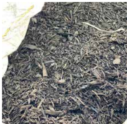
Figure 5. Rubber flakes recovered from the processing of used tires
