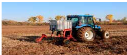
Figure 9. In first plan soil is tillage with new subsoil breaking the hardpan and inoculate microorganisms, in second plan soil was plowed with a mould board plough
