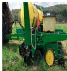
Figure 5. John Deere 7000 planter lateral equipped with granular and liquid fertilizer- lateral view
