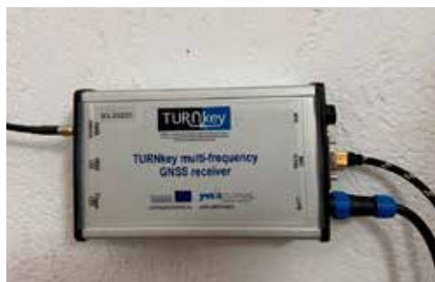
Figure 3. Multi-frequency GNSS receiver fixed on the wall
