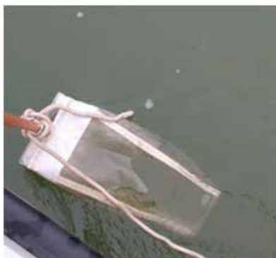
Figure 1. Sampling of plastic particles from the Danube water
