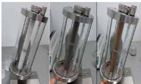
Figure 4. Determination of viscosity using a Hoppler ball viscometer
