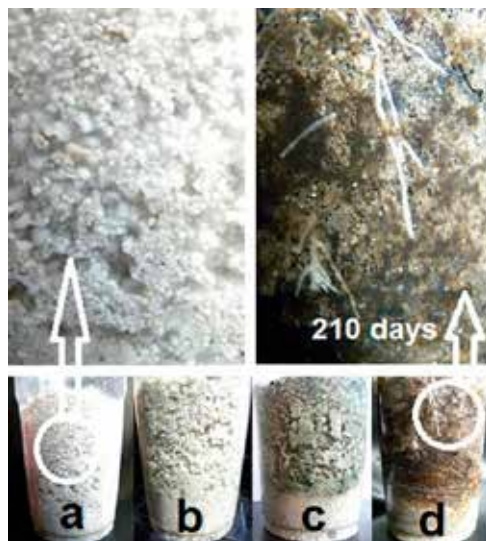
Figure 9. Bioassay pots with (a) bioaugmented expanded perlite; b) bioaugmented expanded perlite, after 61 days; c) bioaugmented expanded perlite and plants influence, after 136 days, and d) after 210 days
