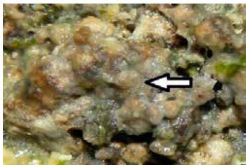
Figure 3. Microbial biofilm on expanded perlite granules, under the action of the consortium
