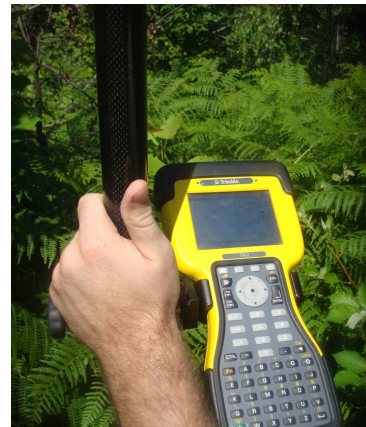
Figure 3. Positioning of details with the GPS system through the RTK method
