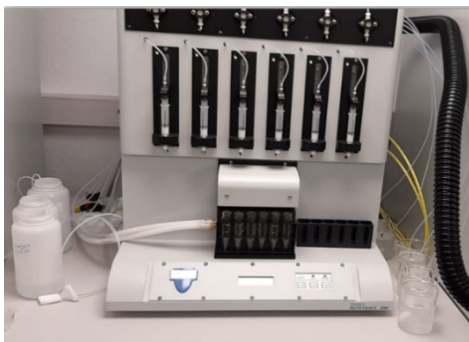
Figure 2. Extraction of pharmaceuticals from water samples
