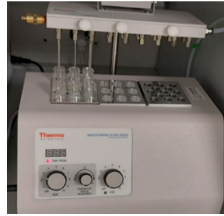
Figure 3. Concentration of eluate under a N 2 flow
