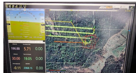
Figure 3. Image footprint and flight path mission created for the aerial survey
