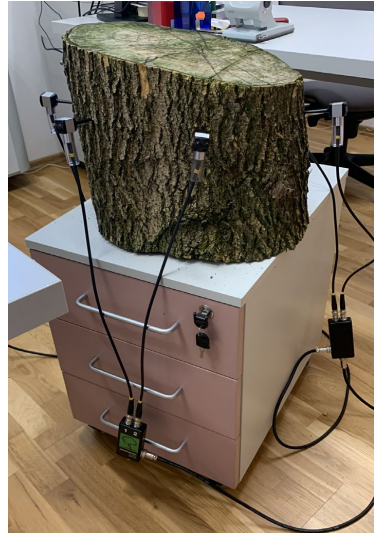
Figure 3. Sound velocity measurement
