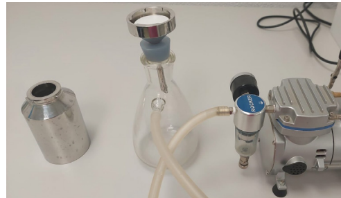
Figure 3. Collection of microplastics on filter paper
