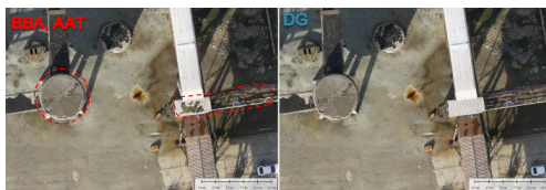
Figure 9. Suspended buildings: differences between classical and LIDAR orthorectification
