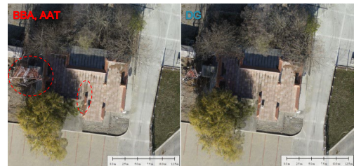
Figure 5. Comparison between classical (left) and on LIDAR data (right) orthorectification
