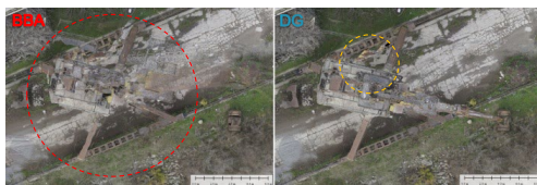
Figure 10. Industrial machinery: differences between classical and LIDAR orthorectification
