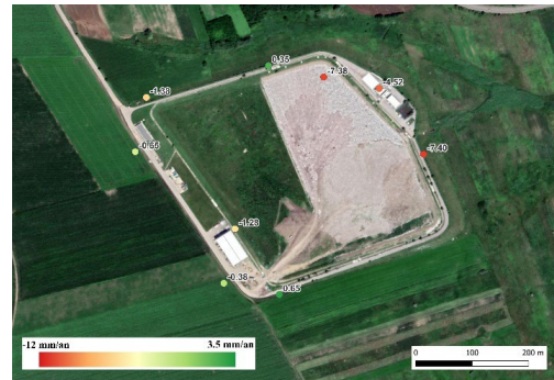
Figure 9. Overall mean displacement velocities (2016-2021) for the persistent scatterers of the Victoria landfill
