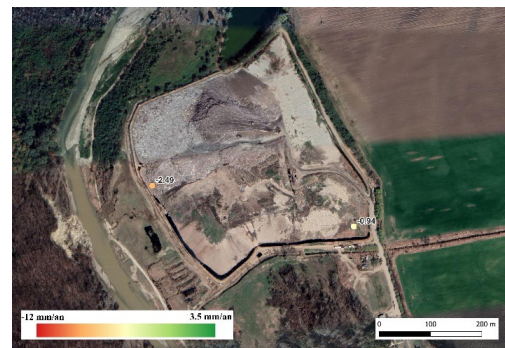
Figure 14. Overall mean displacement velocities (2016-2021) for the persistent scatterers of the Boldești landfill
