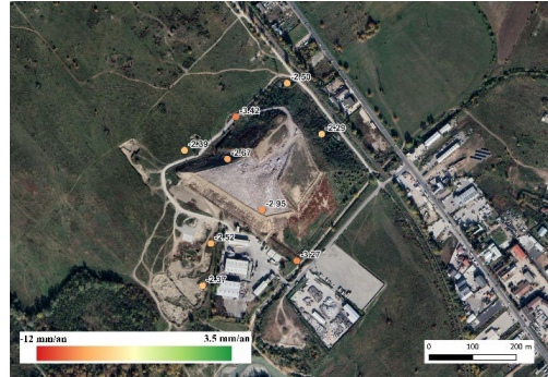
Figure 17. Overall mean displacement velocities (2016-2021) for the persistent scatterers of Aninoasa landfill
