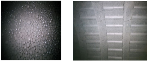
Figure 5. Balls distribution and self-sorting shields (detail) - chamber II
