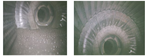
Figure 1. Aspects at the entrance to the mill - material level and cascade armours for chamber I
