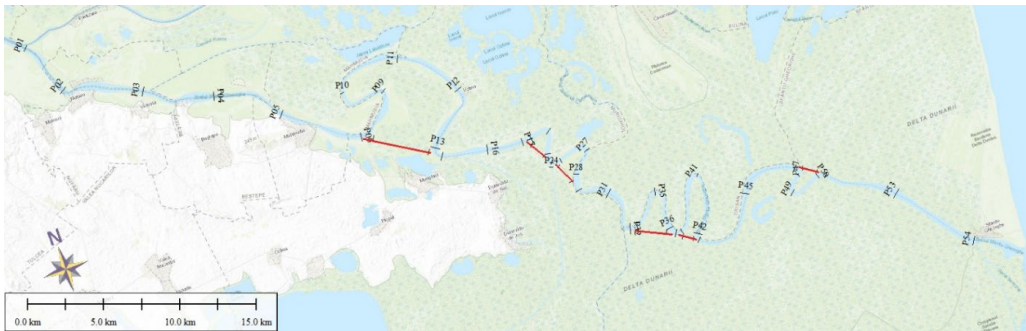
Figure 1. The St. George branch with the position of the investigated cross-sections. The lines in red represent the artificial canals of the rectified meanders (Global Mapper v17)
