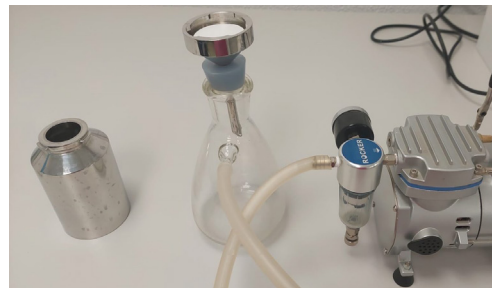
Figure 3. Collection of microplastics on filter paper
