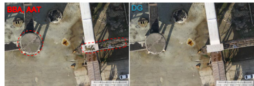
Figure 9. Suspended buildings: differences between classical and LIDAR orthorectification
