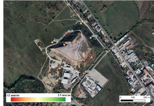
Figure 17. Overall mean displacement velocities (2016-2021) for the persistent scatterers of Aninoasa landfill
