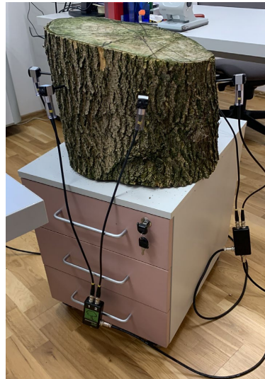
Figure 3. Sound velocity measurement
