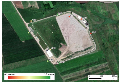
Figure 9. Overall mean displacement velocities (2016-2021) for the persistent scatterers of the Victoria landfill
