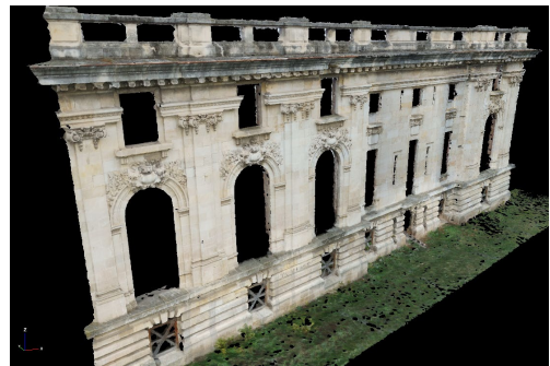
Figure 12. Hybrid 3D model - LIDAR and optical data - 3DF Zephyr
