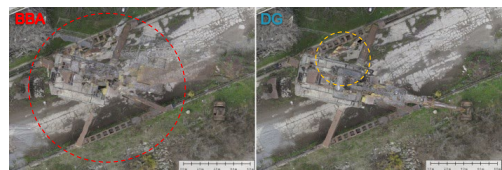
Figure 10. Industrial machinery: differences between classical and LIDAR orthorectification
