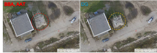
Figure 8. Telecommunication antennas: differences between classical and LIDAR orthorectification
