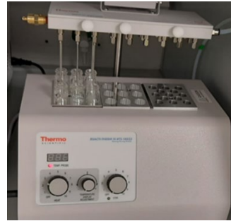
Figure 3. Concentration of eluate under a N 2 flow
