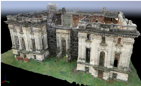
Figure 10. 3D modelling of the Little Trianon Palace based on lateral and vertical images - PIX4D Mapper
