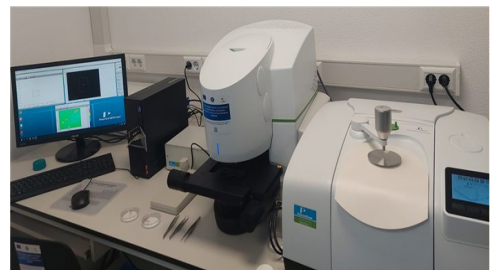
Figure 4. Micro-FT-IR analysis of microplastics
