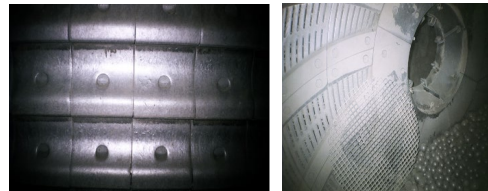
Figure 3. Cascade shields (detail) and slots in the partition wall with ventilation ring (detail) - chamber I
