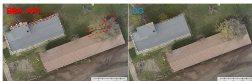
Figure 7. Buildings and vegetation: the improvement brought by orthorectification based on LIDAR data
