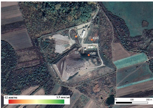
Figure 15. Overall mean displacement velocities (2016-2021) for the persistent scatterers of the Titu landfill
