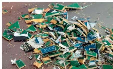
Figure 2. Printed circuit boards subjected to the shredding process
