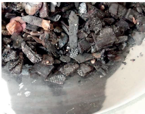
Figure 8. Printed circuit boards after melting
