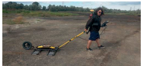
Figure 6. Georadar acquisition data with 100MHz antenna
