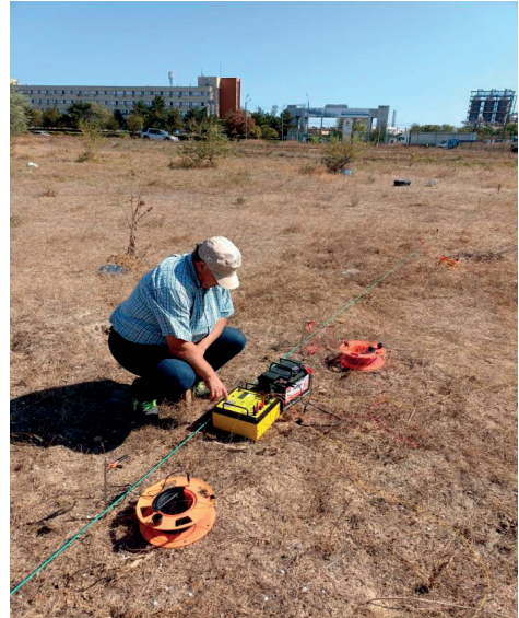
Figure 2. Geoelectric data acquisition using Ministing system from AGI
