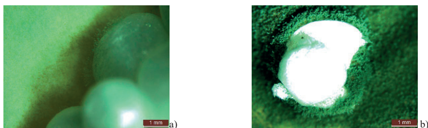
Figure 7. Appearance of the expanded polystyrene sample exposed in an environment contaminated with Penicillium notatum spores: a) after 2 days of exposure; b) after 6 days of exposure
