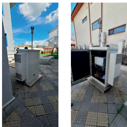
Figure 2. The temperature-controlled box where all air quality requirements were deployed for consistency of data (removing temperature-driven drifts from data series)
