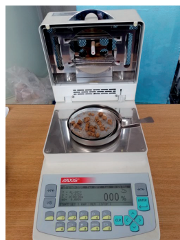
Figure 2. Drying wool pellets with thermobalance Axis-100
